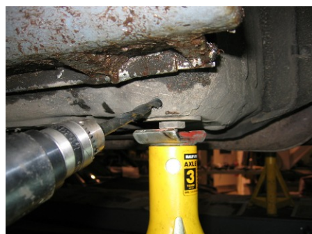
Drilling a front jack point
