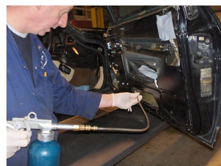
Injecting Waxoyl under high pressure into door cavity...
