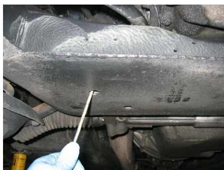
Injecting the front subframe
